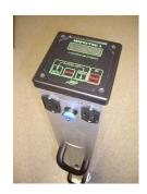
The deflectometer can be used in design, construction, maintenance and quality control of buildings, subdivisions, roads, railways and other environments to measure elastic modulus of unbound or partially bound material, including asphalt, granular aggregation base, base layers, soil, concrete etc.
