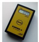
RADON-3 is a handheld alpha ( $\alpha$ ), beta ( $\beta$ ), gamma ( $\gamma$ ) and X-ray radiation detector that is designed to monitor and measure equivalent dose rate of radiation. The device is very sensitive and can detect even small sources of radiation.
