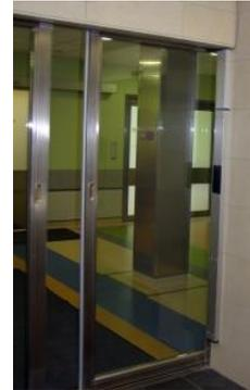
RADMONITOR is a stationary door-mounted gamma ( $\gamma$ ) and X-ray radiation detector system that is designed to monitor and measure equivalent dose rate of radiation. The system is ideal in institutions to prevent individuals from bringing radioactive elements in or out of buildings, in hospital radiation therapy units to ensure that patients don't leave the area until it's safe to do so, and in other applications.
