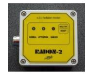
RADON-2 is a stationary alpha ( $\alpha$ ), beta ( $\beta$ ), gamma ( $\gamma$ ) and X-ray radiation detector that is designed to monitor and measure equivalent dose rate of radiation.
