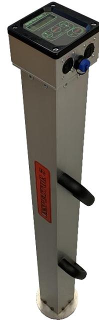
A built-in GPS unit determines and stores the exact location of the measurement, which can later be graphically displayed in Google Maps. INSPECTOR-5 is rated IP65 under the international IEC 60529 standard and is splash and dust proof.
