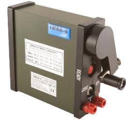
ERNA-4 is a medium energy blasting machine that comes with a built-in three point line tester. It uses a hand generator and the operator does not need an external power supply or batteries. The blasting machine is portable, compact and lightweight, and can easily be operated by a single person.
