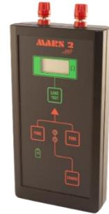
The integrated line tester measures the detonator line resistance to identify short circuits, breaks in the blasting line or circuits with excessive resistance prior to the blast. For safety reasons, the line tester current is limited to 1mA.
